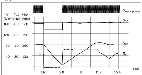
$U_{DC}$  = Intermediate circuit voltage of the drive,
