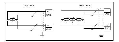
WARNING! IEC 60664 requires double or reinforced insulation between live parts and the surface of accessible parts of electrical equipment which are either non-conductive or conductive but not connected to the protective earth.
