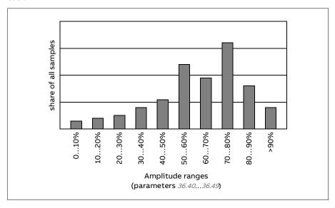
Amplitude logger 1 is fixed to monitor motor current, and cannot be reset. With amplitude logger 1, 100% corresponds to the maximum output current of the drive ( $\prime_{max}$ ). The maximum output current values are listed in the section
