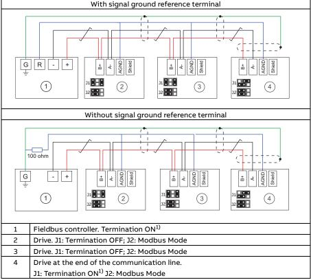
1) Note: The drive at both ends on the fieldbus must have termination set to ON.
