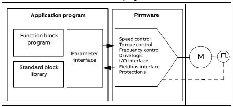
The firmware program performs the main control functions, including speed, torque and frequency control, drive logic (start/stop), I/O, feedback, communication and protection functions. Firmware functions are configured and programmed with parameters.
