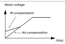
In vector control, no IR compensation is possible or needed as it is applied automatically.
