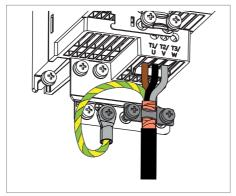
5. Twist the motor cable shield into a bundle, mark it with yellow-green and connect it to the grounding terminal.
