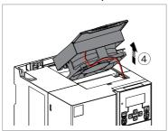
5. Install the new fan into the fan cover. Make sure that the air flow is in the correct direction. The air flows in from the bottom of the drive and out from the top of the drive.
